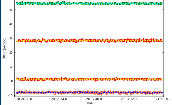
Typical antenna pointing offsets for VLA as a function of time
